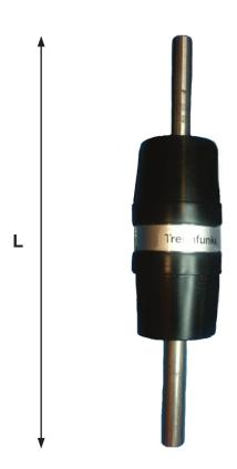
SG closed spark gap can handle lightning discharge currents of 100 kA (8/20  $\mu$ s). Connection 2 x A2 M10.
