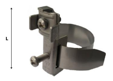
GS A2 grounding strip provides an earthing junction between Ø 17 - 48 round pole or cable and 1 x 16 mm² - 2 x 25 m² grounding cable.
